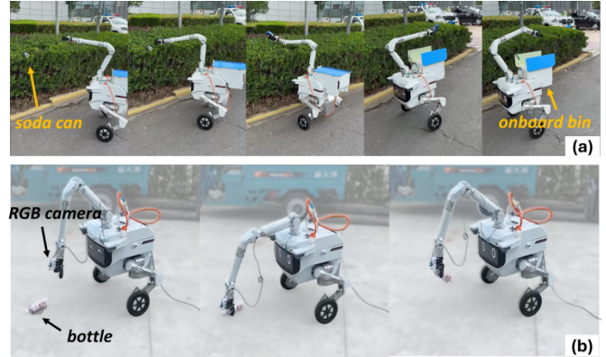
Fig. 1: Real-world deployment. The robot tracks velocity commands to reach the target position, and the robotic arm performs manipulation tasks via two different control methods. (a) The robot grasps a roadside soda can and place it into the onboard bin via human remote teleoperation. (b) The robot picks up a plastic bottle from the ground via the finetuned VLA model GR00T N1 [4], details are in VI-D.
