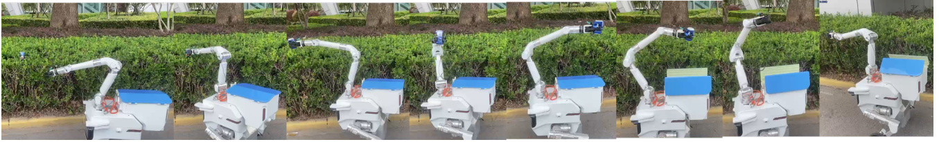
Fig. 6: One demonstration of outdoor waste collection task. The robot navigates to the target location, executes continuous and complex manipulation motions to place the waste into the onboard bin, and then continues to the next target.
